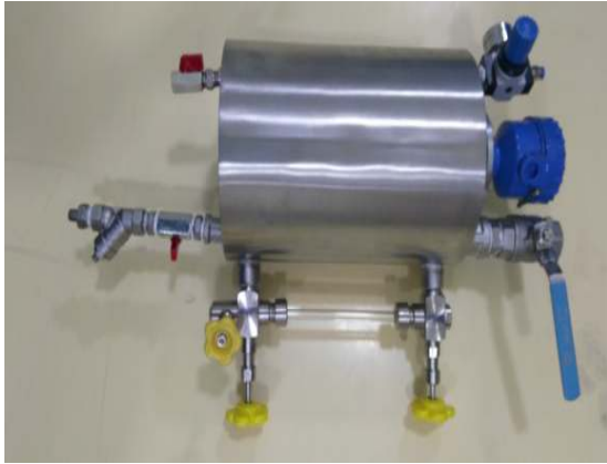
PLC Controlled Lubrication System
