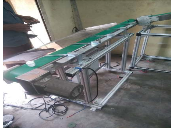
L Conveyor with Auto Collection Trays
